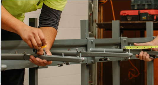
Front-mounting design for easy fab shop gang mounting
